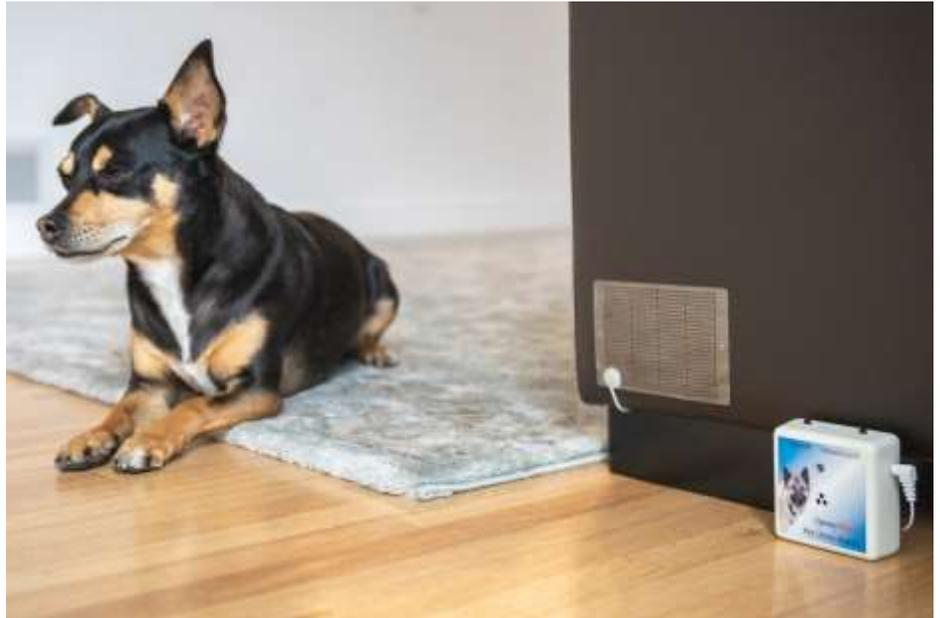
On vertical surfaces such as walls the sensor must be flush with mounting surface. Place it where dripping urine will run over the face of the sensor. On flat or horizontal surfaces, secure it in place with double sided adhesive or tape. Minimize loose hanging cable to discourage pet from playing with it. Tape it down if necessary, especially to hide from curious dogs.
